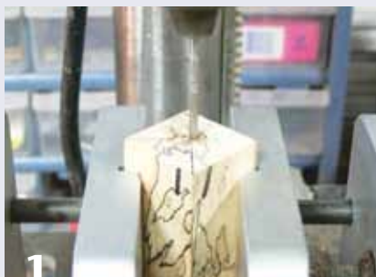
1 Drill the hole where the brass tube will be inserted. The brass tube strengthens the endgrain-to-endgrain joint.
