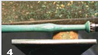
4 Measure the diameter of the crochet hook to achieve the correct size. Use a Knit-Chek and calipers.
