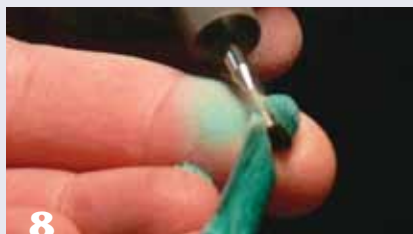
8 Use a cylinder-shaped diamond carving bit to make sure the burn marks are removed from the hook area.
