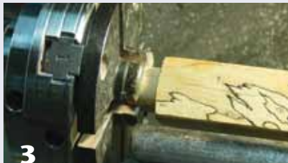
3 Leave a ¼" (6 mm) gap between the shoulder of the turning blank and the shoulder of the chuck jaw.
