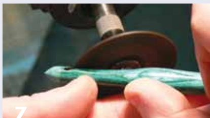
7 Cut the hook part of the crochet hook using a fiber cut-off wheel held in a rotary device.
