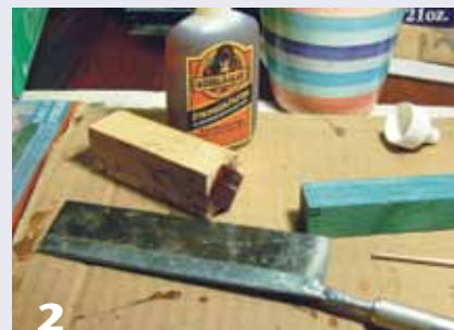
2 Use Gorilla polyurethane glue to secure the brass rod into the holes. There are three sections to this crochet hook.
